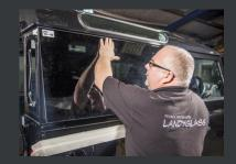
Find the edge trim in your kit, this covers all metal edge sides and back quaters. When fitting you will need to pull the trim away on the corners for the glue to adhere to the metal work correctly. Do not forget to prime the corner nice and close to the edge.
