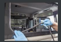
Fit the edge trim supplied onto the metal edge around the window of the Land Rover. Use the wipe pouch from kit to clean the body before priming.
