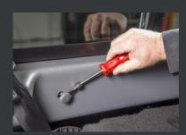
Remove all four handles at the top of the trim by tapping screws under the covers. You will now need to remove the fir tree fitting at the bottom of the panel.
