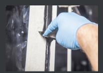
Refit the trim inside, replacing any broken clips. When the glue is dry you can trim the very edge of the glass to five a clean finish. You can wash off the next day, or use glass cleaner to clean the alass.
