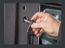
Begin with removing the black cover on the seat bolt, then using a 17mm socket, remove the seat bolt. We now need to remove both of the fir tree clips, the first clip can be found just above the seat bolt as shown in the photo; remove these with the trim removal tool
