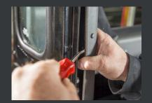
Grab your trim removal tool and start unclipping the trim, there are two clips on either side, both of which will need to be removed.
