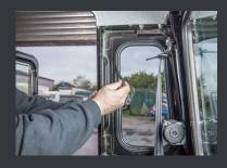
We now need to remove the rear quarter, to start remove the rear window lace; when completed remove the rubber and the glass. You will need to be careful when removing the glass because heavy hands can cause shattering, push the glass inwards and wear gloves.
